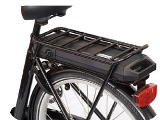
To disconnect the battery, unlock the battery lock with the battery key clockwise. Then remove the battery from the controller box by pulling the handle at the bottom of the battery.
